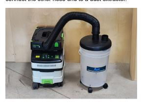
4. Thread the coupler 63 mm on the second flexi hose and insert it into the side hole of the lid. Use another coupler 63 mm or wire clip 63 mm and connect the other hose end to a power tool or router table.
